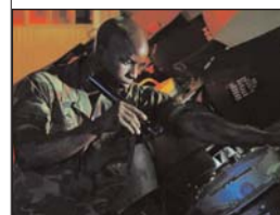
ABOVE, Top: Turboprop engine mechanic Staff Sgt. Carla West performs an inspection of a newly installed tailpipe assembly on an EC-130H Compass Call aircraft. Bottom: Air Force Senior Airman Brandon Benson uses a flashlight to inspect the interior of a C-130 barrel assembly for cracks during a routine check. HAWKEYE helps support complex electronic and mechanical systems.
