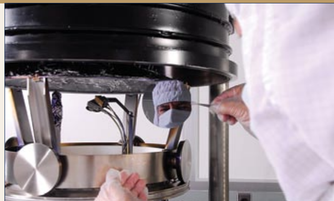
Carefully maintained and updated, a 50-year-old vacuum evaporator is still applying coatings in a Georgia Tech Research Institute clean room.
