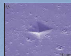
ABOVE: At top is an indentation made in stainless steel by a Vickers indenter. At bottom is an indentation made with the same indenter and load into boron carbide.
