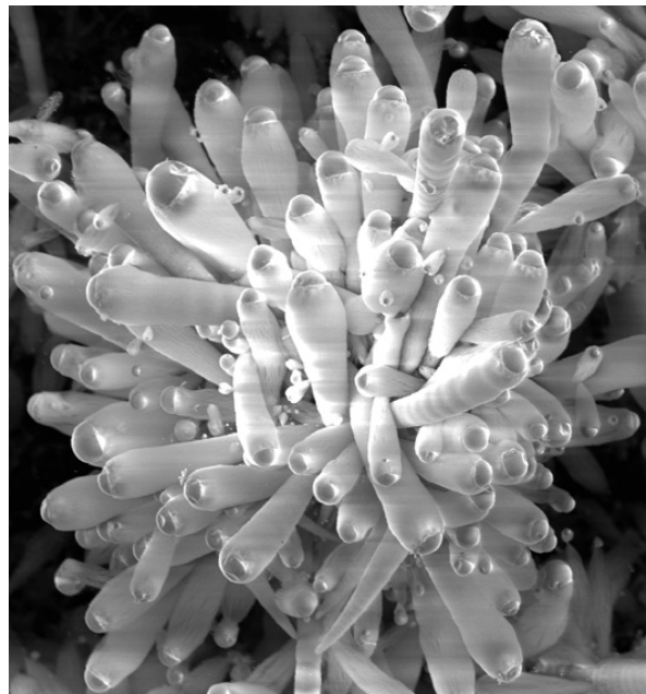
Carrot-shaped structures were produced from bundles of aligned nanowires grown on a silicon substrate. Each carrot contains hundreds of thousands of nanowires.
